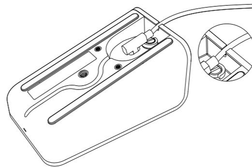
A. Connect the USB-C cable to the Dock using the 90 degree connector side. The cable should be pushed into the slot at the rear of the Dock.
