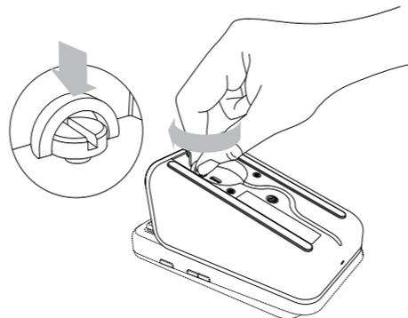
To lock the Reader to the Dock place the Reader aligned with the Dock on a flat surface. Push downwards on the D ring bolt to engage with the Reader nut threads and turn clockwise until tight. When locked fully the Reader should have little to no movement on the Dock.
