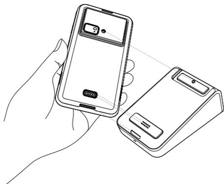
To charge the Reader, place on the Dock ensuring that pogo pins are mating with contact points, lock nut mates with locking bolt and lower slot mates with hook.
