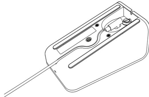
B. When the cable is to exit the front of the Dock, the cable should be pressed into the channel.
